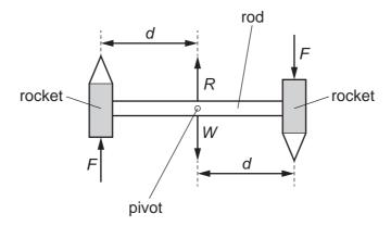
Each rocket exerts a force of magnitude F on the rod at a perpendicular distance d from the pivot. The forces exerted by the rockets are always in opposite directions.
