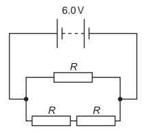
The total power dissipated in the resistor network is 24 W.
