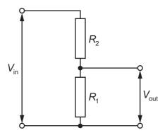
Which changes to  $R_1$  and  $R_2$  will increase the value of  $V_{out}$ ?
