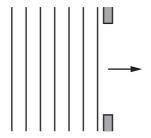
Some diffraction of the water waves is observed.
